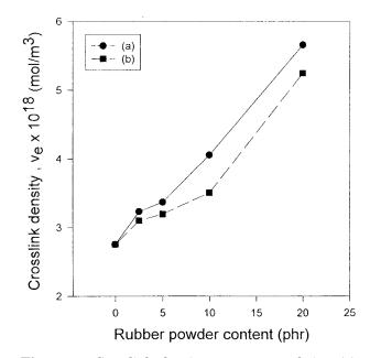
**Figure 7** Crosslink density vs. content of tire: (a) untreatment; (b) chemical treatment.
