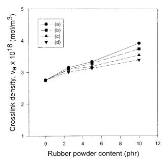
**Figure 8** Crosslink density vs. content of tire with different microbial treated days: (a) treated for 5 days; (b) treated for 10 days; (c) treated for 20 days; (d) treated for 30 days.
