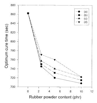
**Figure 6** Optimum cure time vs. content of tire with different microbial treated days: (a) treated for 5 days; (b) treated for 10 days; (c) treated for 20 days; (d) treated for 30 days.
