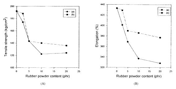
**Figure 3** (A) Tensile strength vs. content of tire. (B) Elongation vs. content of tire: (a) untreatment; (b) chemical treatment.
