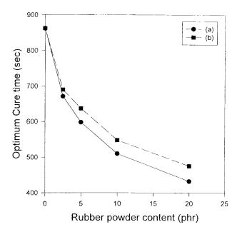
**Figure 5** Optimum cure time vs. content of tire: (a) untreatment; (b) chemical treatment.
