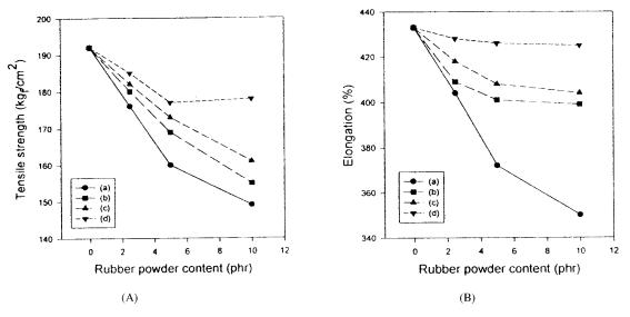
**Figure 4** (A) Tensile strength vs. content of tire with different microbial treated days. (B) Elongation vs. content of tire with different microbial treated days: (a) treated for 5 days; (b) treated for 10 days; (c) treated for 20 days; (d) treated for 30 days.
